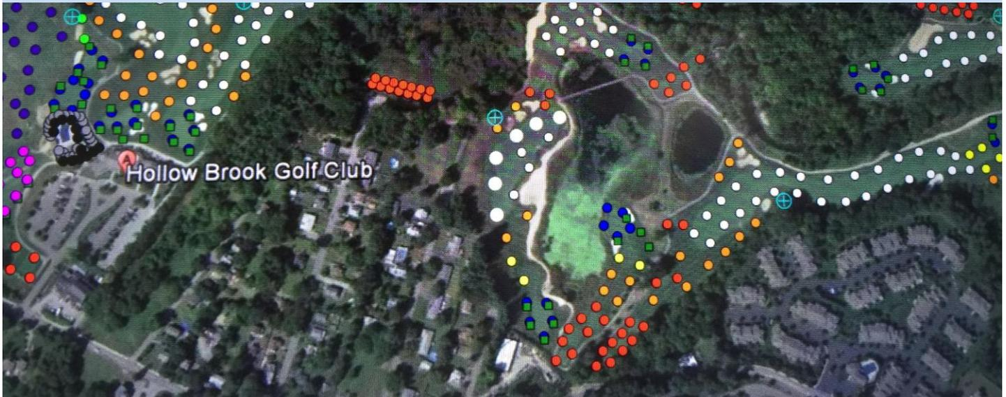
*Interactive map of every sprinkler head on the golf course. The user can select a sprinkler head to run or can visualize which ones will run. The highlighted white dots are heads that are within an instant program created just for high sides of fairways, which need more water than the flat surfaces.*
